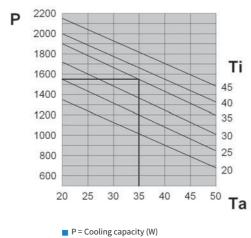
P = Cooling capacity (W)
