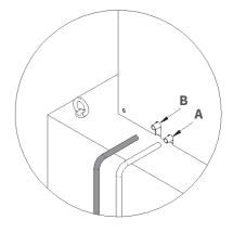
For maximum protection of the electrical components, DEK units are equipped with dual condensate outlets in the electrical cabinet.
