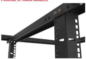
Rack angles are sold in pairs that are RU marked on all sides. One side is tapped 10-32 while the other side is square hole (.375 x .375 in.). Both sides are spaced per EIA universal standard. Rack angles may be assembled in either tapped or square-hole configuration. Rack angles and mounting brackets are formed from heavy gauge steel and are polyester powder painted low-gloss, RAL 9005 black. All hardware and brackets are included for assembly into cabinet.
